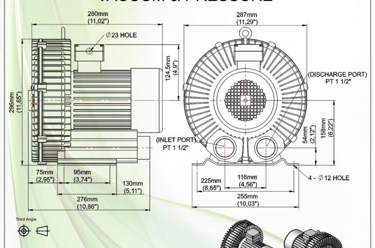
\* The allowable tolerance of dimension is ± 5mm
